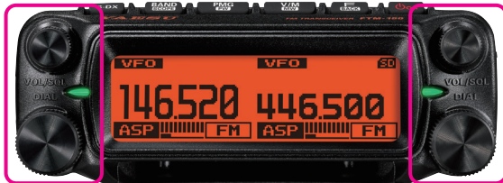
Controls for each band are placed independently on the left and right
