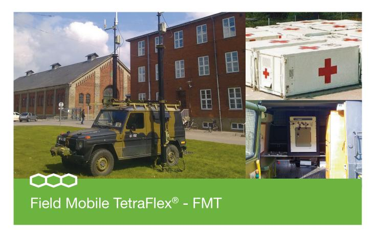
DAMM's Field Mobile TetraFlex® (FMT) solution is a fully functional two-carrier TETRA communication system. Housed in a 19" modular cassette, it has been specifically designed for field deployable solutions. Its convenient size and form factor mean that it can be easily built-in to trucks, cars, containers or other mobile units.
